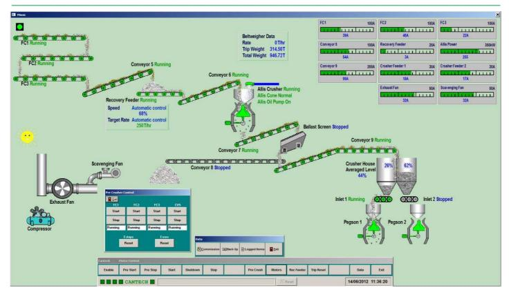
The continuing need to improve operating efficiency and product quality whilst increasing plant output and improving employee health and safety are all met by using Cantech's latest-generation CS-2000 crushing and screening control system. This operates any or all of the primary, secondary and tertiary crushing processes remotely from a central control room or weighbridge office.
